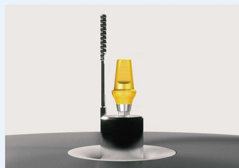
Purpose-built Jig for Abutment photoactivation
